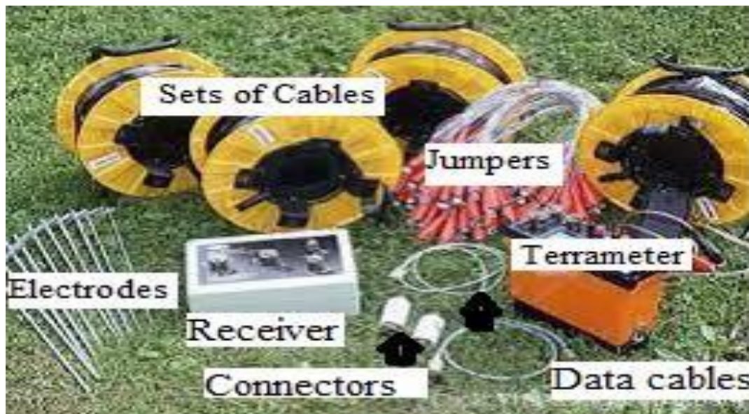
Figure 3.2: Pictorial view of the ABEM LUND Imaging system and its various components (Modified after: Reynolds, 2011)
