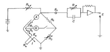
Figure 2.14: Constant Current Anemometer Bridge Circuit
