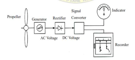
**Figure 2.12: Signal Flow Diagram**
