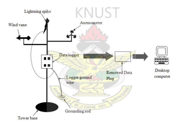
Figure 3.1: Layout of Experimental Set-Up
