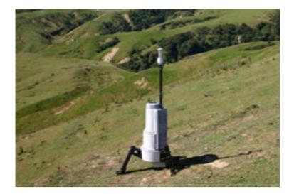
Figure 2.18: ZephIR Laser Anemometer. Source: Wind Measurement International
