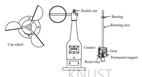
Figure 2.8: Three-Cup-Wheel Wind-Path Anemometer Source: JMA, 2010
