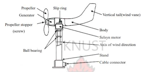
Figure 2.11: Generator-Type Propeller Anemometer
