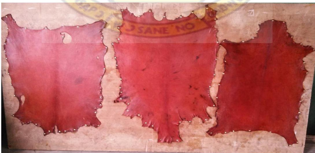
Plate 3.10: Stretched leather on the wooden board
