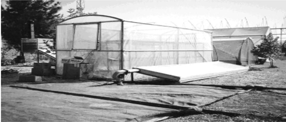
**Plate: 2.2 Solar tunnel dryer**
