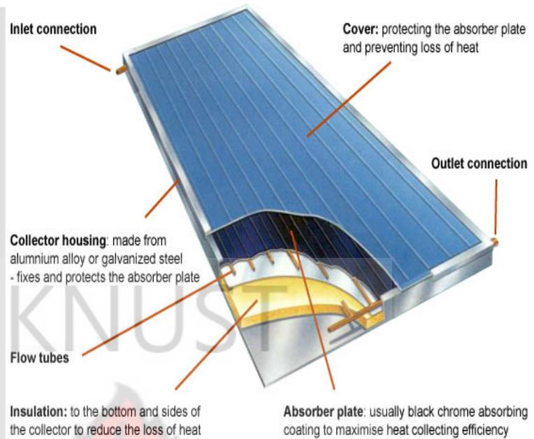
Figure 2.4 Glazed solar collector. Source [9]
