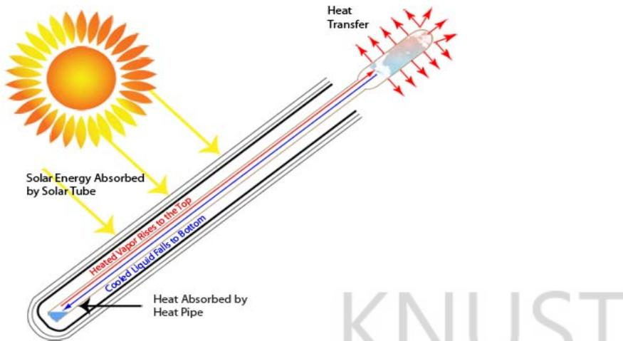
Figure 2.5 Evacuated tube collectors. Source [10];
