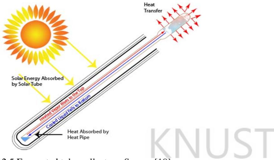
Figure 2.5 Evacuated tube collectors. Source [10];
