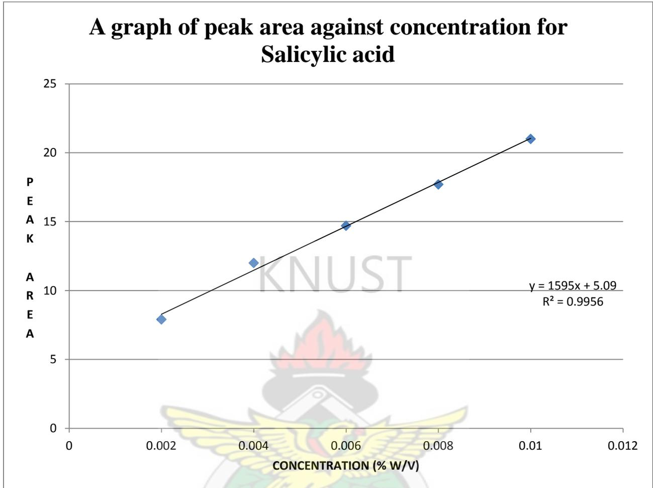
Figure 24: Calibration curve for salicylic acid
