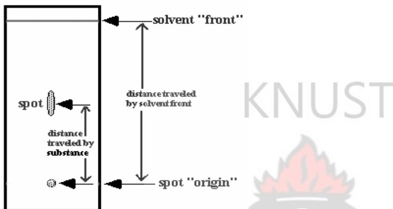
Figure 4: TLC plate showing the distances travelled by the spot and the solvent.
