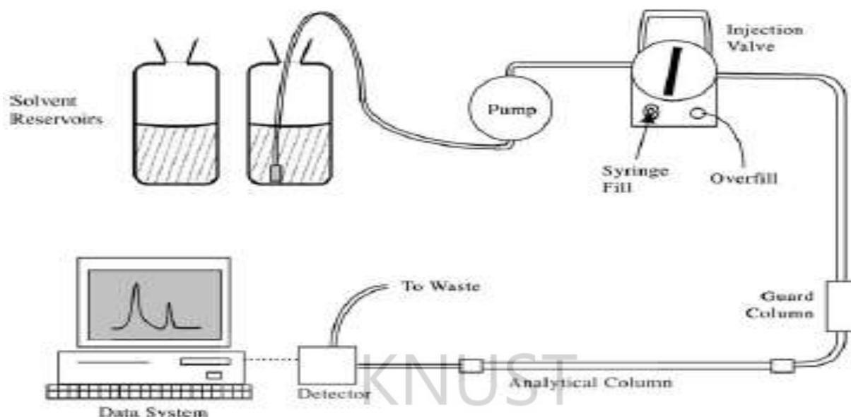
Figure 5: A graphic representation of an HPLC system.
