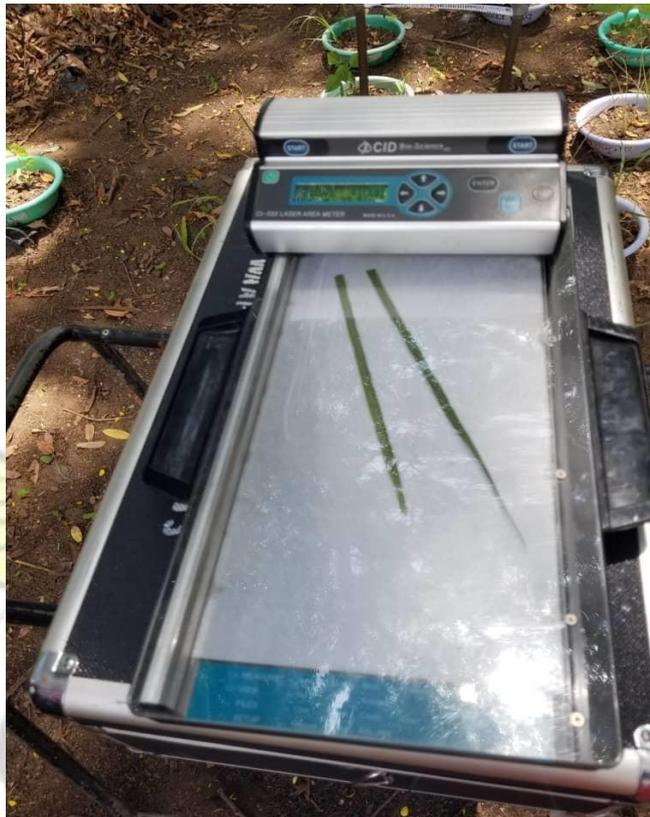
**Plate 3.2. CI-202 Portable laser leaf Area meter**
