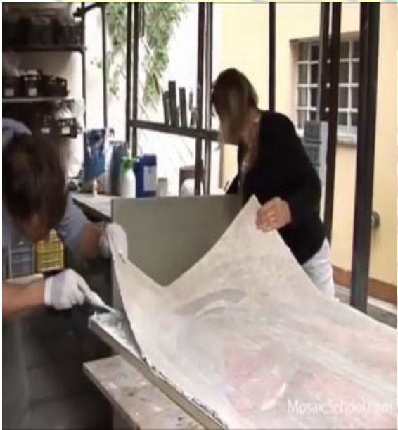
Figure 2. 21: work is removed from the sticky surface
