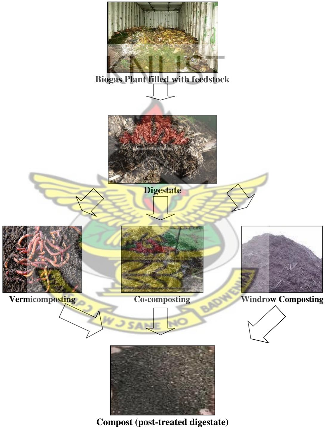
**Fig. 3.2: Digestion and composting processes**
