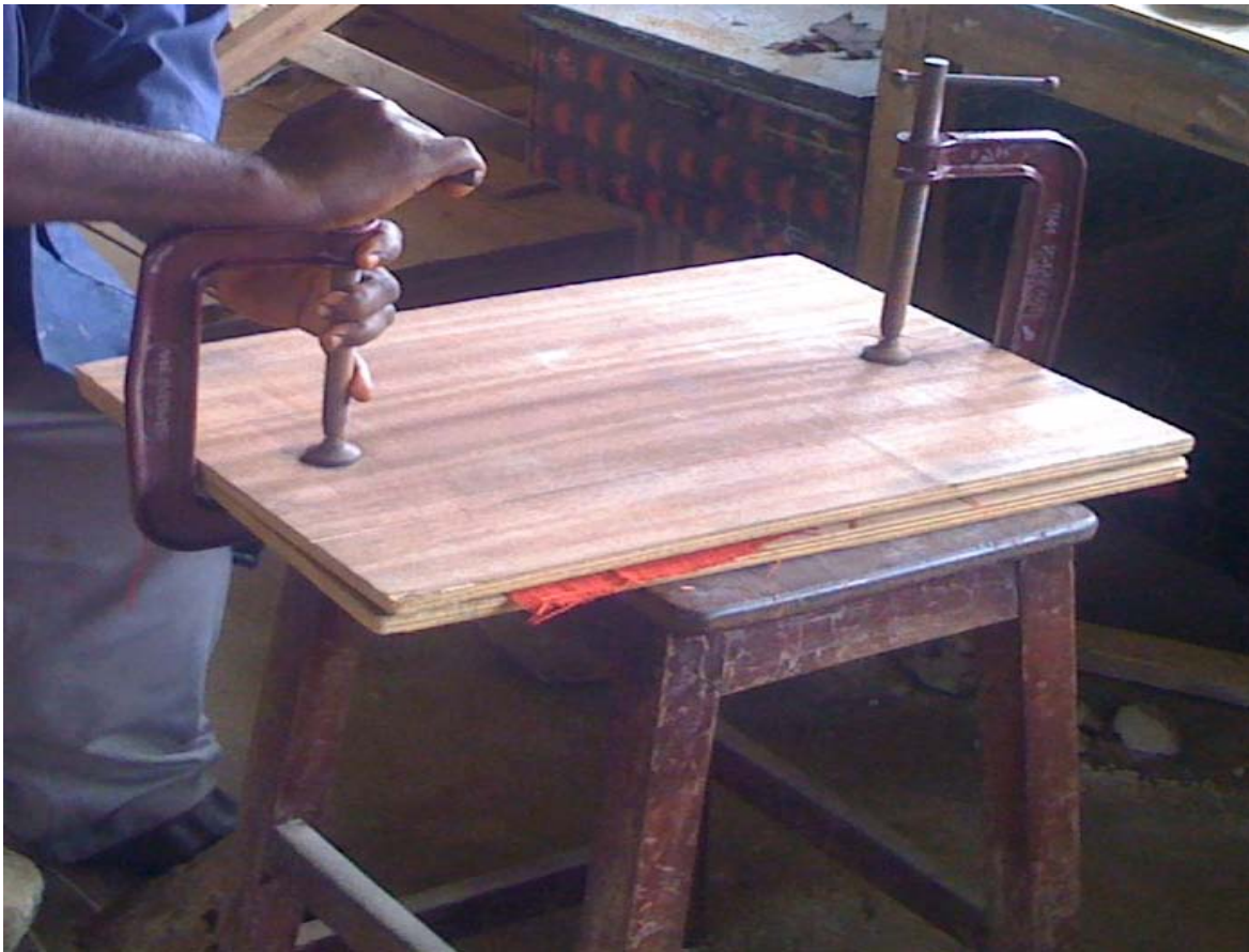
Plate 12: Pressing wet support
