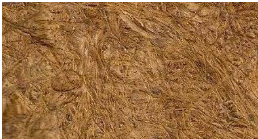
Fig 3. Sample of Support from Teak Tree Bark
