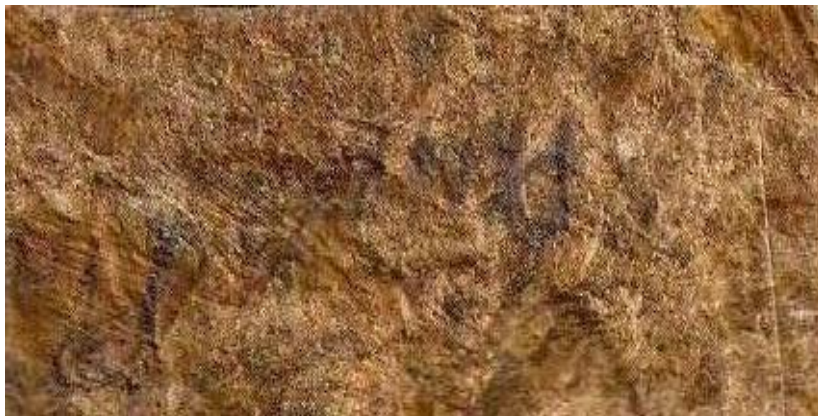
Fig7. Sample of Support from Pineapple Leaves
