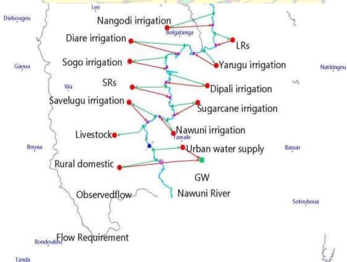
Figure 3.3 Schematic view of the river and modelled parameters in WEAP
