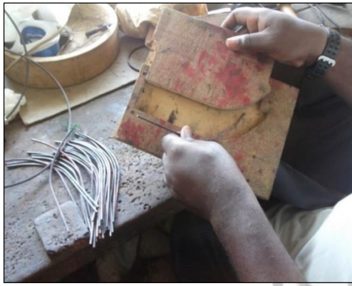
Fig. 3.29: Forming of 'half u' stakes Fig. 3.30: Formed rings with mould
