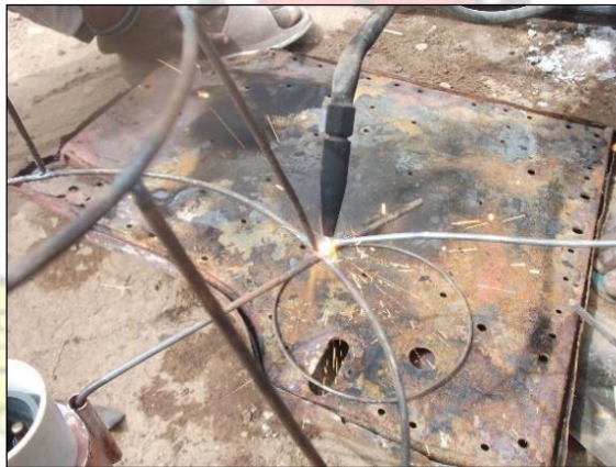
Fig. 3.79: Brazing the shade support
