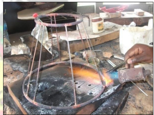
Fig. 3.73: Soldering of the stakes between the rings
