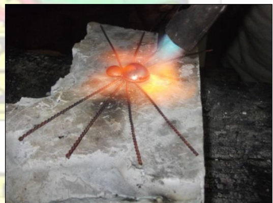
Fig. 3.12: Soldering the spider's legs
