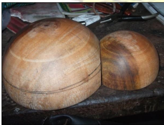
Fig. 3.53: Wooden mould for the forming of the spider
