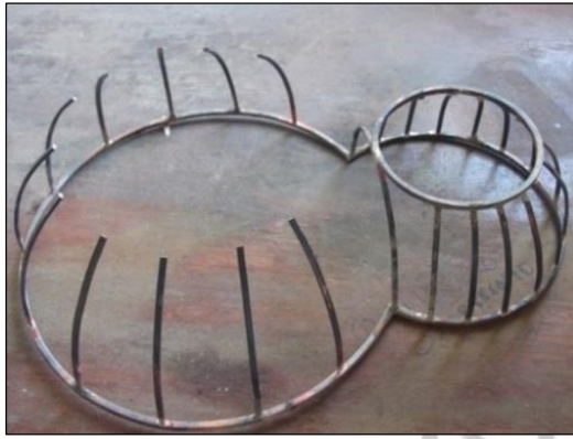
Fig. 3.55: Soldered warp stakes
