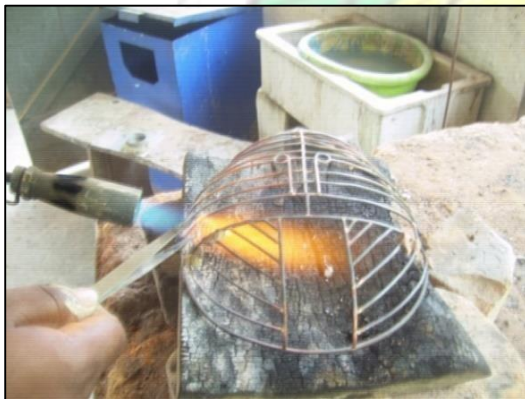
Fig. 3.14: Soldering the armature
