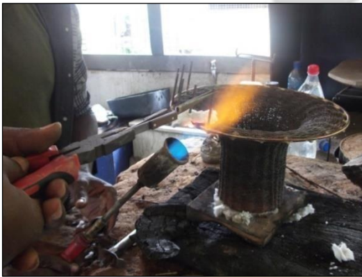
Fig. 3.33: Soldering the stakes that form section B
