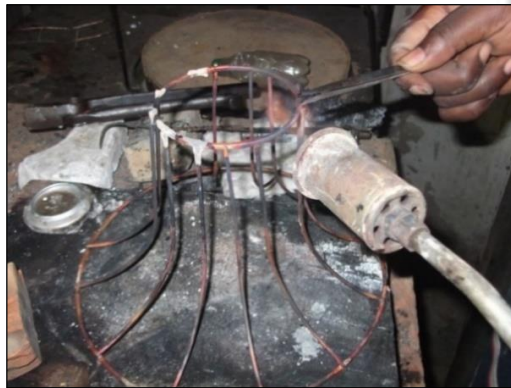
Fig. 3.31: Soldering the stakes around the rings
