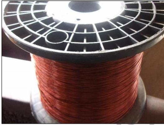
Fig. 3.5: 0.64mm copper wire
