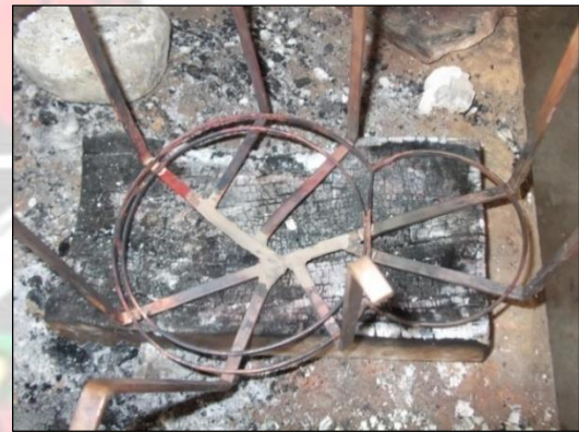
Fig. 3.60: Soldering of legs to the base
