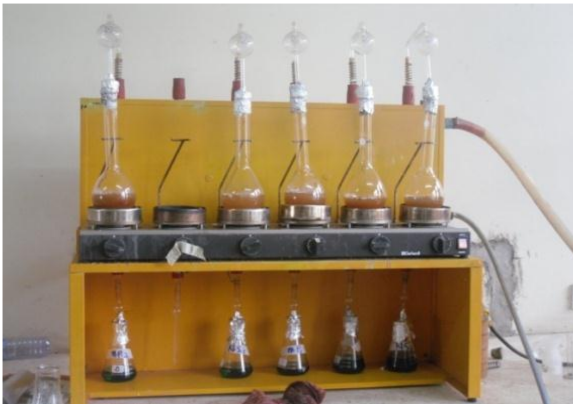
Figure 3. 3 Sample distillation using the Kjeldahl Distiller
