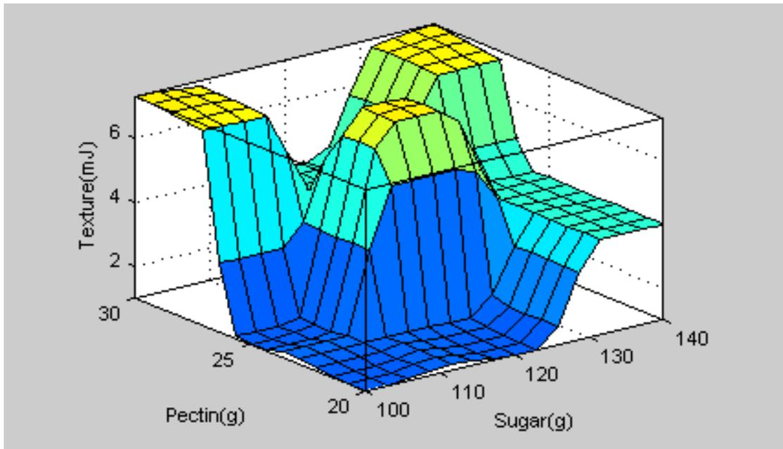
**Figure 4.3a: Surface plot showing effect of sugar and pectin on jam's texture quality**
