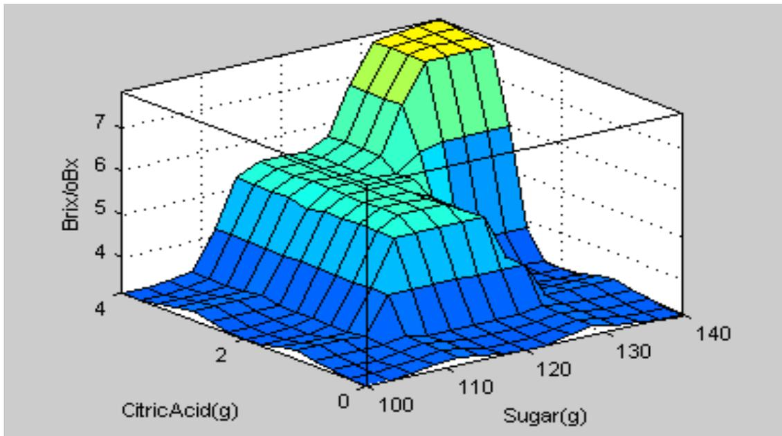
**Figure 4.4b: Surface plot showing how sugar and citric acid affects brix quality of jam**
