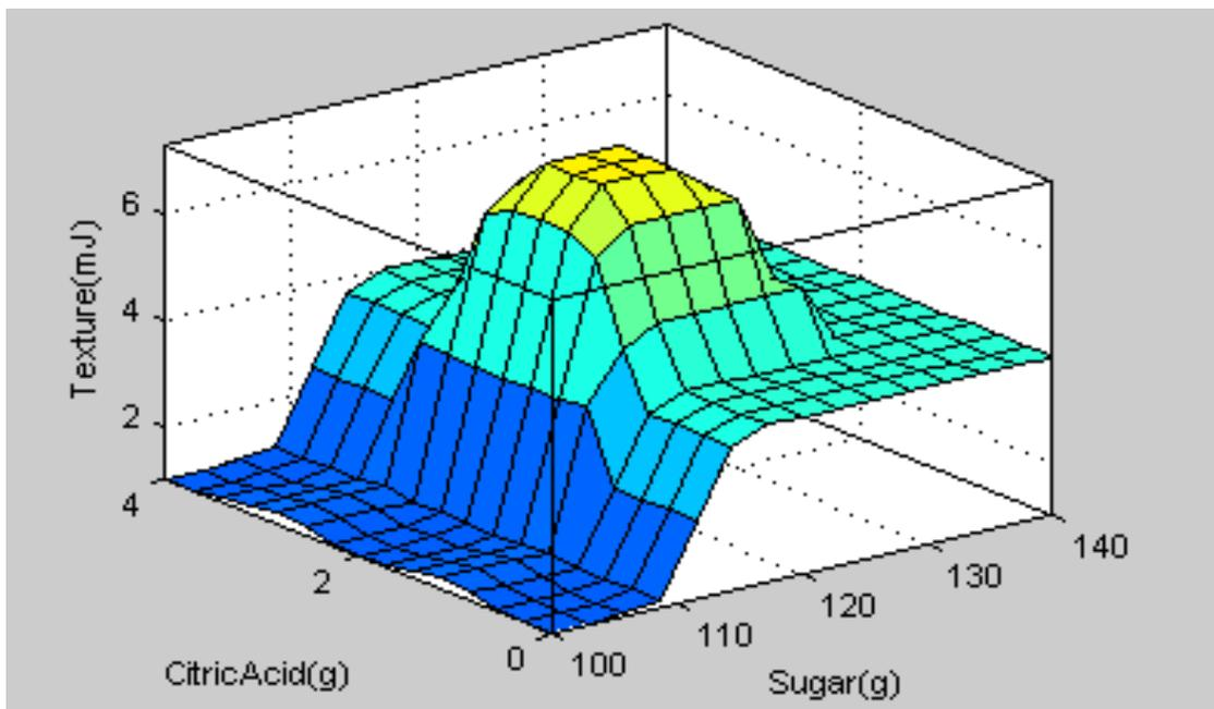
**Figure 4.3b: Surface plot showing effect of sugar and citric acid on jam's texture quality**
