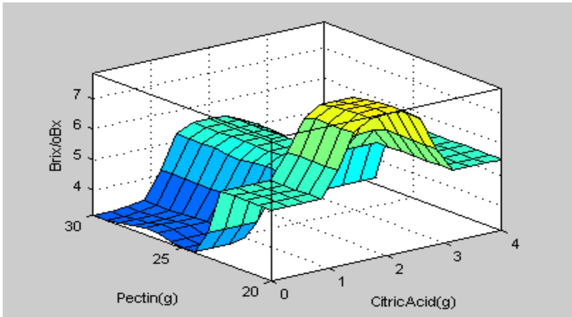
**Figure 4.4c: Surface plot showing how sugar and citric acid affects brix quality of jam**
