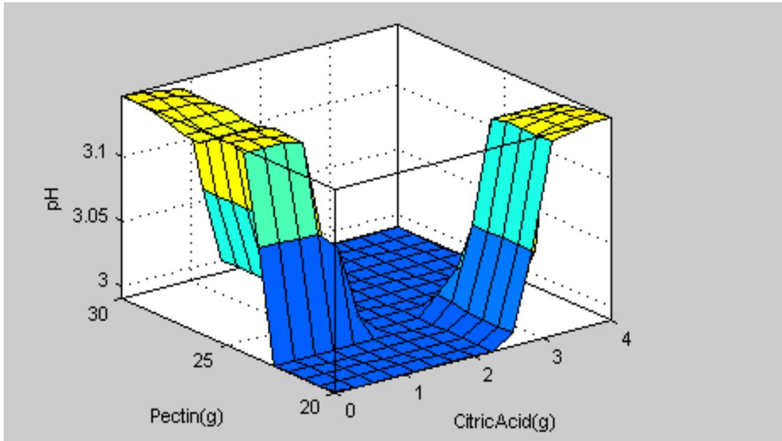
**Figure 4.2c: Surface plot showing effect of citric acid and pectin on jam's pH quality**
