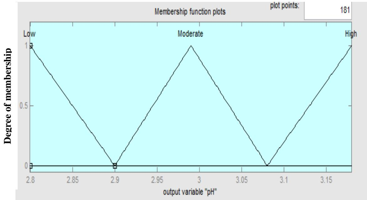
**Figure 3.2a: Membership function plots of ‘low’, ‘moderate’ and ‘high’ jam pH output**
