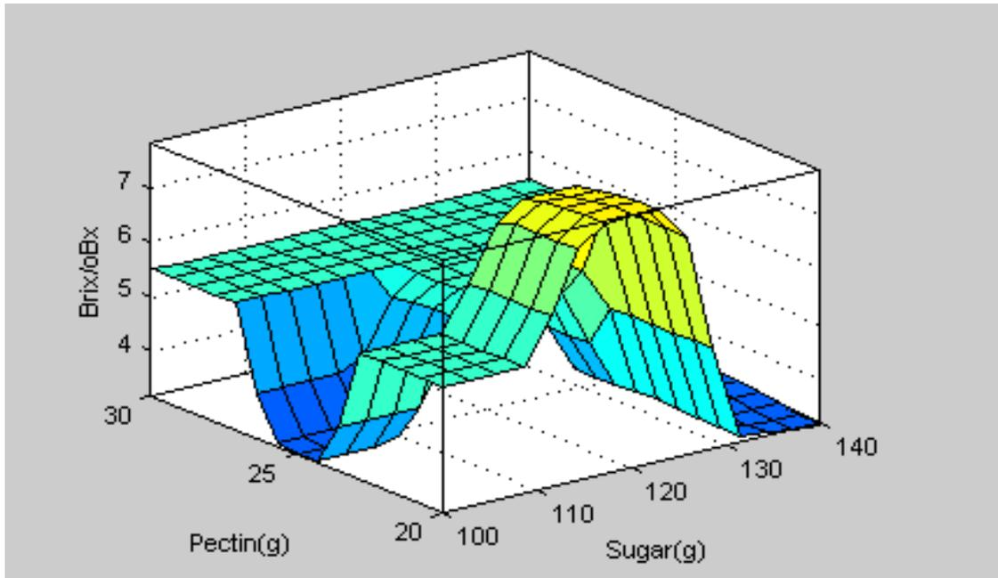
**Figure 4.4a: Surface plot showing how of sugar and pectin affects brix quality of jam.**
