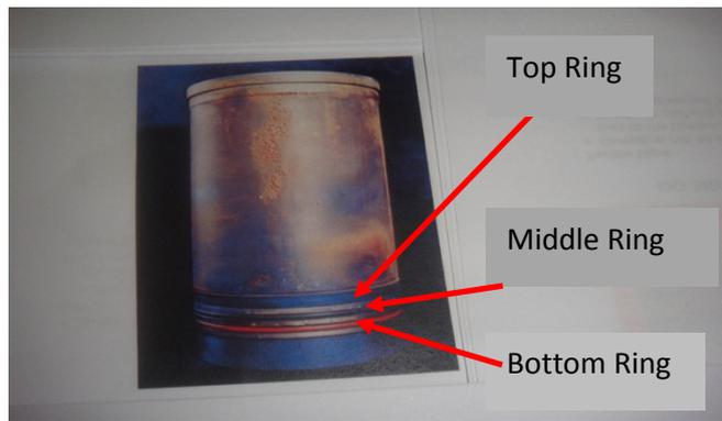
**Figure 4.7: Wet type liner with the various types of seals**
