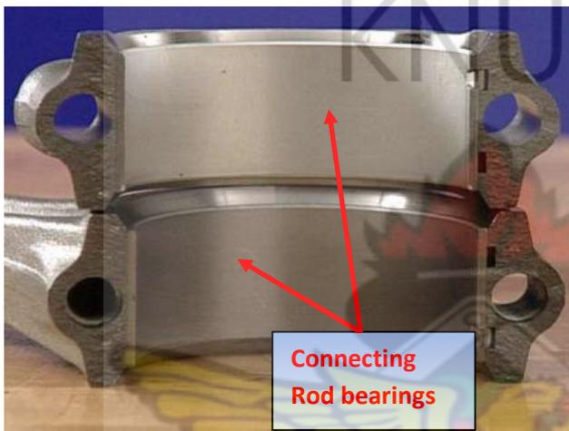
**Figure 4.9: Connecting rod fitted with connecting rod bearings**
