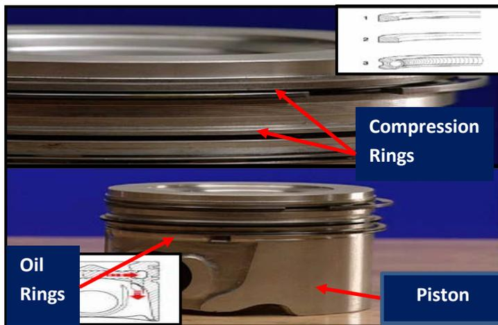
**Figure 4.8: Positioning of the oil and compression rings**
