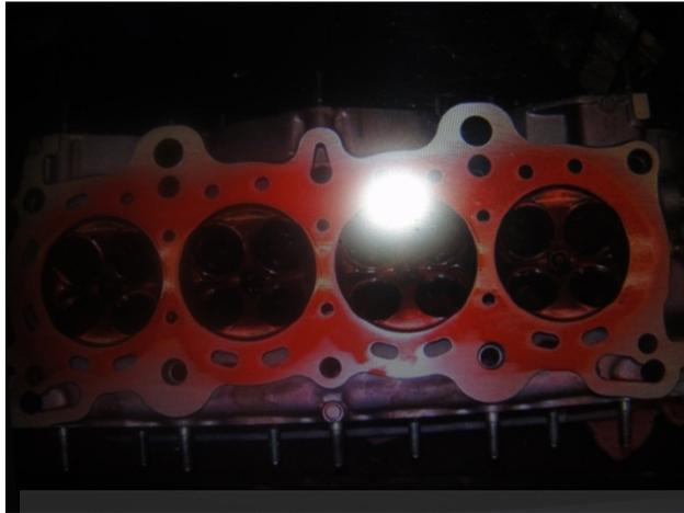
**Figure 4.3: Cylinder head test showing bright red lines to aid in crack detection**
