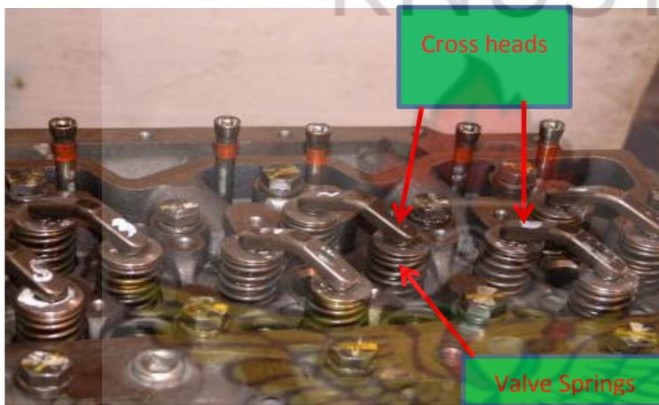
**Figure 4.15: Cross Heads with valve springs**
