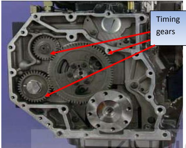
**Figure 4.12: Timing gears of a heavy duty engine**
