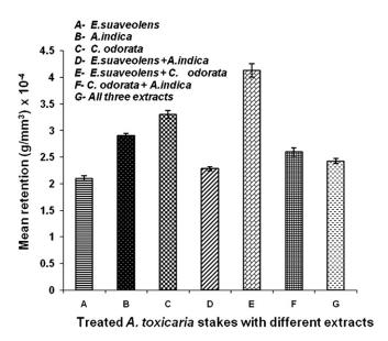
**Fig. 1.** Mean retentions for the different extracts impregnated into *A. toxicaria* stakes. NB: Bars = standard errors.
