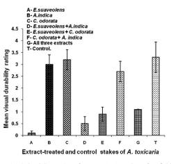
Fig. 2. Mean visual durability ratings for A. toxicaria stakes after field exposure. NB: Bars = standard errors.
