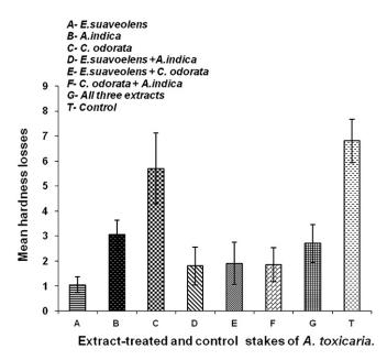
**Fig. 4.** Mean percentage hardness losses in *A. toxicaria* stakes after field exposure. NB: Bars = standard errors.
