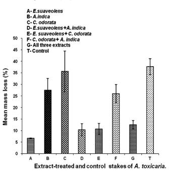
Fig. 3. Mean percentage mass losses for A. toxicaria stakes after field exposure. NB: Bars = standard errors
