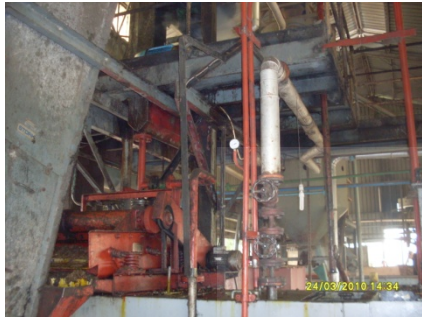
Plate 4.29 Pipes interfering circulation paths (Adansi Oil Mills)
