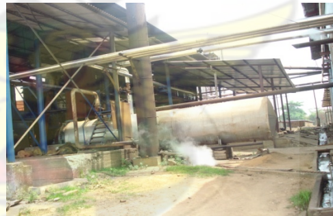
Plate 4.15 Pipes conveying steam to sterilizers (Juabeng Oil Mills)
