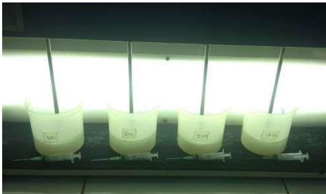
Plate 5: Set-up for batch adsorption experiments
