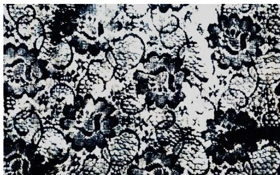
Fig., 14: Discharge effect produced all over the dischargeable fabric with lace material
