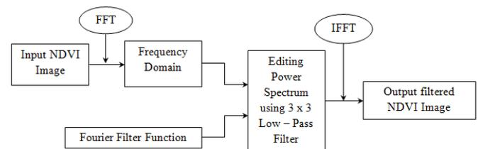
Figure 2.2: Diagram Summarizing the FFT application.
